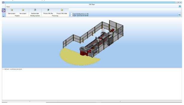
$\mathbf{CNCPipes}\,$  , interface application between CADMATIC XML files and Transfluid TXT files
